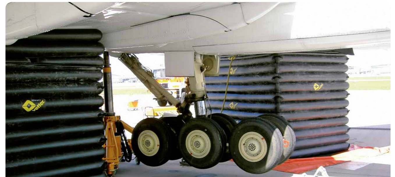
Aircraft Lifting Bags - quick and secure recovery
