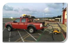
Using a Findlay Irvine MK2 Grip Tester the 100m section was recorded at **0.93**, compared to pre-application grip level of **0.83**
