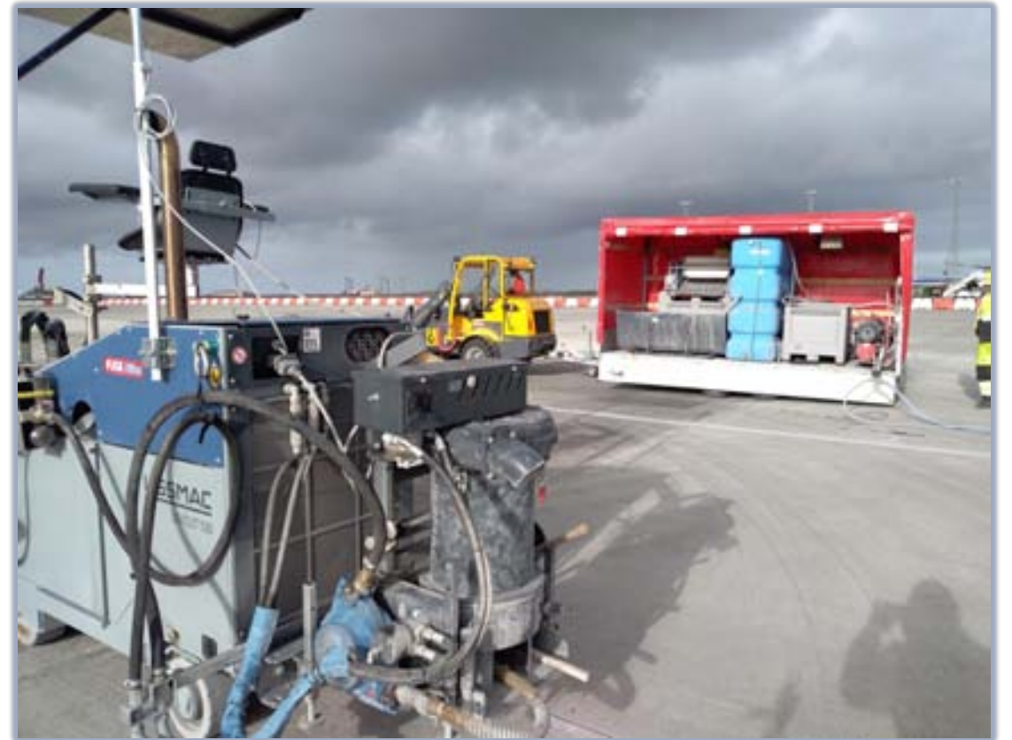
Precision cutting machine connected to a water filtering system, that reduces water consumption from 20.000 liter per day to just 1.000 liter.
