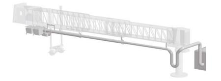
The special construction with flexible outside and inside bearings guarantees a proper adaption of the telescopic tube to axial and lateral movements of the boarding bridge and is furthermore self-supporting over long spans. The gasket designed by IST withstands temperature fluctuations from  $-40^{\circ}$ C to  $+80^{\circ}$ C and is absolutely wear resistant.
