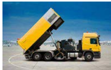
The tank and sound hood can be tilted hydraulically for maintenance purposes and for emptying the waste water tank. This allows easy access to all components – high pressure pump, boost pump, fan, cooler and extractor.
