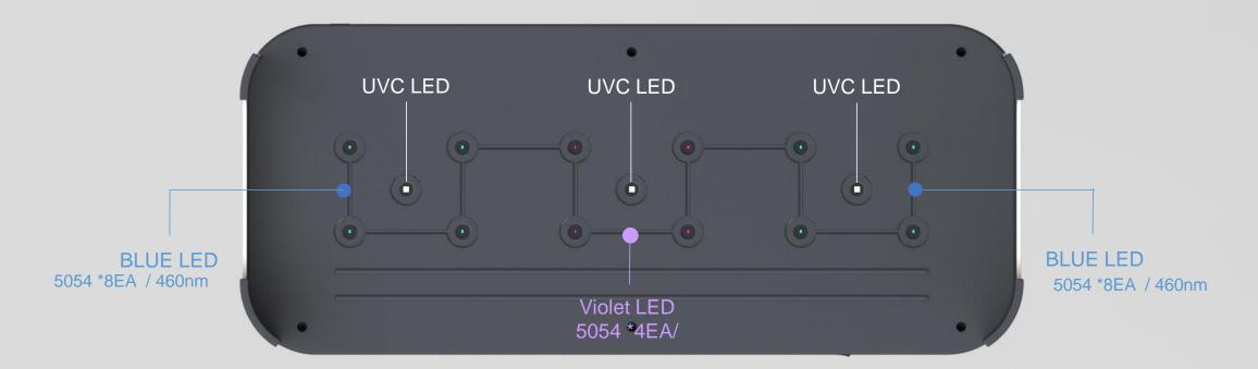
UVC LED 90mW ( 30mW \*3EA ) / 260nm~280nm/ Angle 160° BLUE LED 5054 \*8EA / 460nm Violet LED 5054 \*4EA/ R:620nm G:520nm B:490nm
