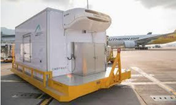
Ground handlers are offering, in more and more airports an expensive active tarmac transport solution that can be a refrigerated truck or a thermal dolly. Those solutions have high extra costs and are powered with gasoline or rechargeable batteries which produce an CO2 emission. In addition, those are special equipment that needs to be maintained and monitored and have a long Return Of Investment.
