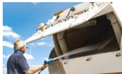
An installed washing device with hose reel, hose and spray gun can be used to clean the tank (after tilting) or the vehicle.
