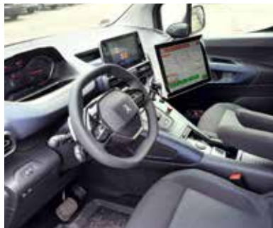
The cabin with the control panel
