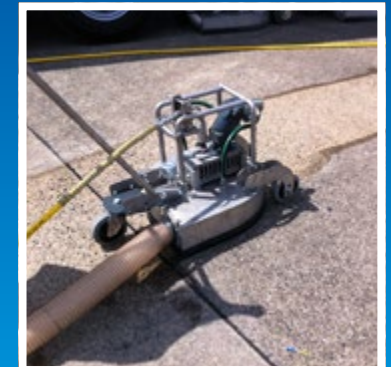
Small inaccessible areas can be handled with the hand cleaner MCD 360 (optional).
