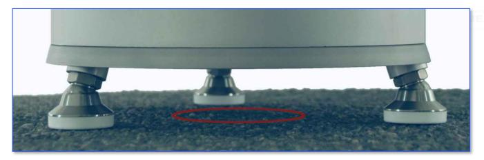
The rotating laser sensor of the ELAtextur scans the pavement surface with a horizontal resolution of 0.2 mm. The circumference of the circular path is 400 mm (according to the sand-patch method).
