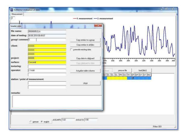
For evaluation and printouts of measurements carried out with the ELAtextur a software has been developed to realize the following visualisation:
