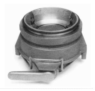
The Meggitt 3-inch bottom loading coupler is designed for the use in bulk plant system where the standard 4 inch API F228 coupler is to large. The F214 coupler mates with F429 adapter and has a unique snap - on pull - off connection action not used on the larger relatives. The coupler is available with 2, 2.5 and 3-inch female pipe threads or a 3-inch TTMA flange.
