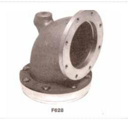
Meggit has a line of delivery hose swivels that provide excellent swiveling characteristics and yet utilize no ball bearings. Seals and bearings used in the F628 swivels are easily replaced facilitating maintenance. Each Meggitt swivel has a main liquid seal, a Teflon bearing and a dust seal to prevent damage to the bearing and main seal from road dirt.
