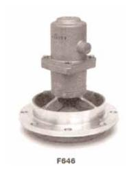
Meggitt F646 Series 5.25 inch vents are designed in accordance with DOT MC306 specifications and will mate with a standard 4-inch TTMA sump ring. The venting capacity is 304,000 cu. ft/hr at five PSI and the cracking pressure is three PSI. The F646 vent is available in air and mechanically operated configurations.
