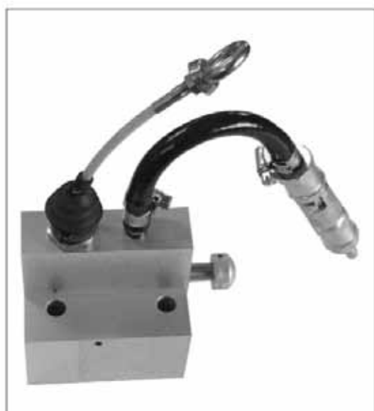
Pneumatically operated pilot valve
