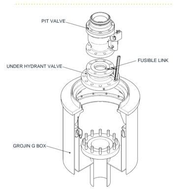
When fitted is operated by rotating the handle, thus opening the flap valve against a bespoke internal torsion spring. The design incorporates an automatic pressure equalisation feature, allowing the valve to be opened easily even when the hydrant is pressurised.
